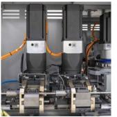
The chain link blank transport passes the chain link to the bending station
