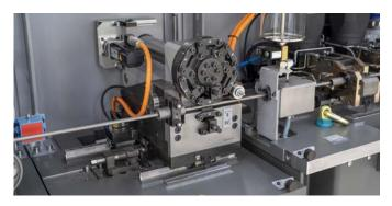
Die forming device and notching device
