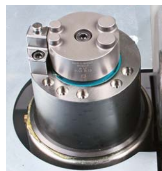
▲ 4-Pin bending tool, type 5
